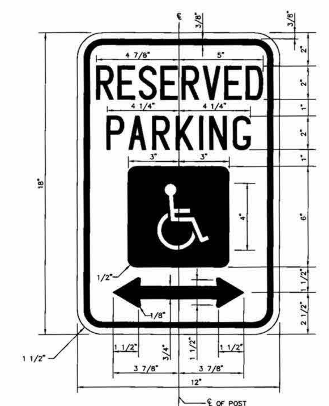
COLORS LEGEND AND BORDER - GREEN WHITE SYMBOL ON BLUE BACKGROUND BACKGROUND - WHITE NOTE: FOR ADDITIONAL INFORMATION, REFER TO SIGN MOUNTING DETAIL, THIS SHEET.
